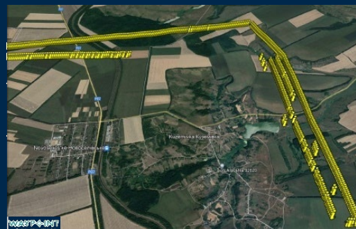
EW causes position gaps & jumps of UAV, rejected by Autopilot
